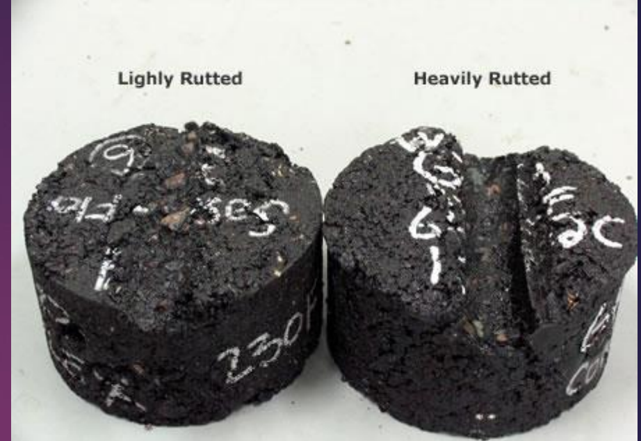
Figure 2: Comparison of a rut-resistant HMA (left) and a rut-susceptible HMA (right) after 8,000 load cycles in the APA.
