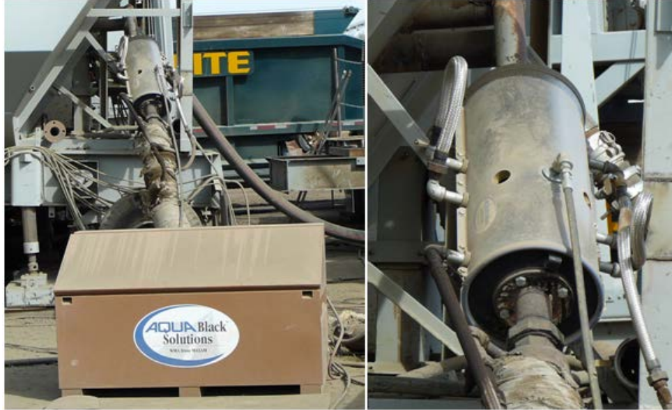
FIGURE 1 Maxam AquaBlack™ WMA System
