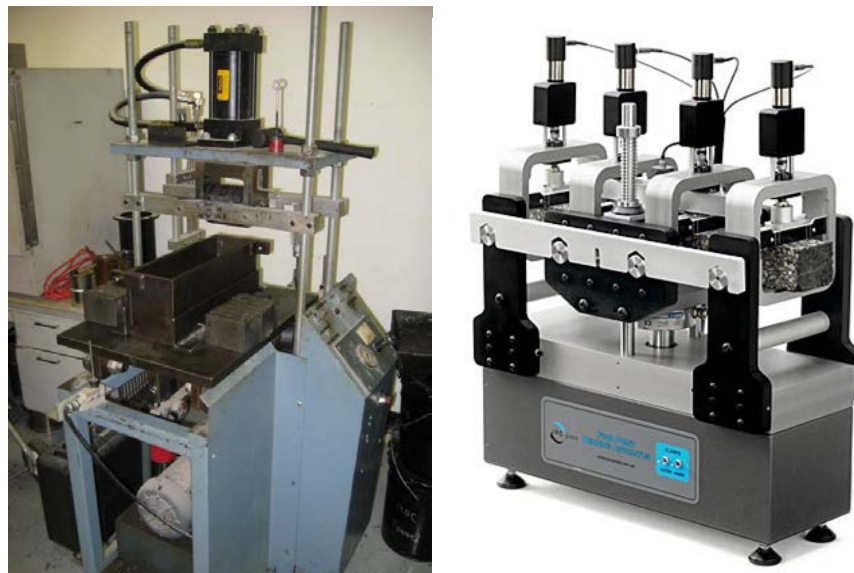
Figure 17 Kneading Beam Compactor (left) and IPC Global® Beam Fatigue Testing Apparatus (right)
