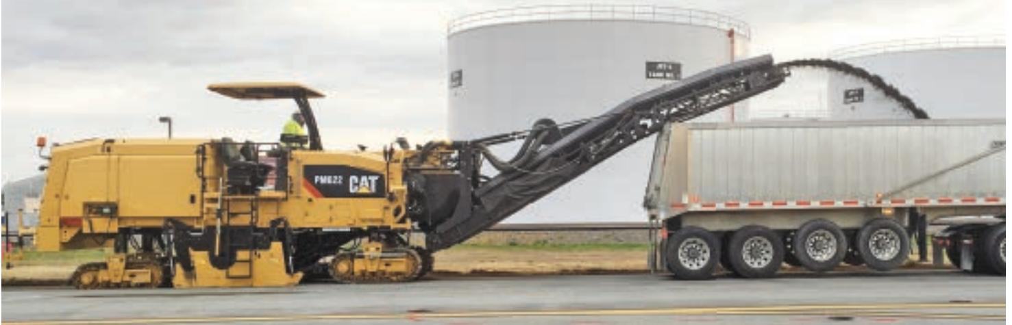
The PM622 is a highly productive, highly maneuverable half-lane milling machine that performs controlled full-depth removal of asphalt and concrete pavements in a single pass.
