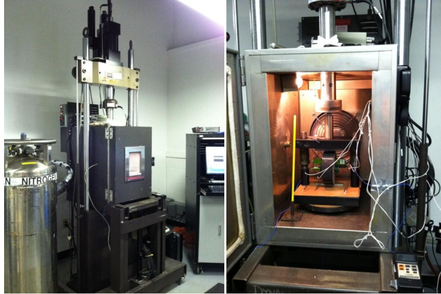
Figure 19 MTS® Load Frame (left) and Specimen Setup for IDT Testing (right)
