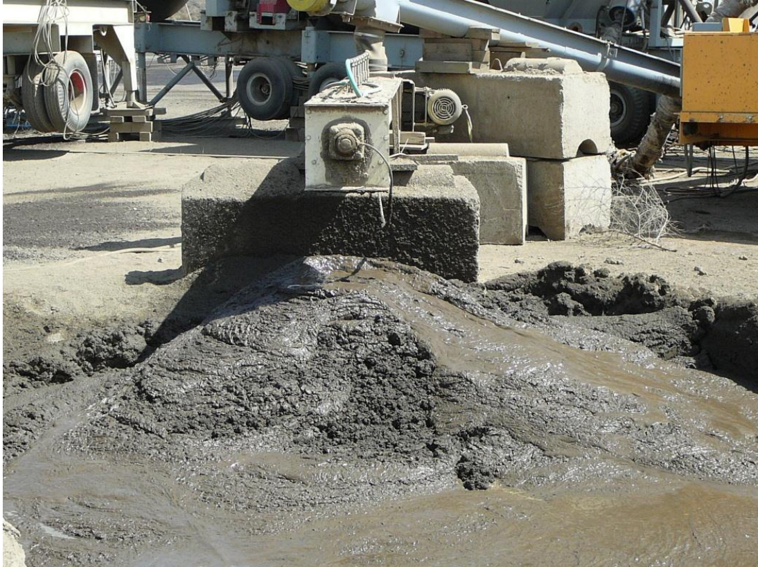
FIGURE 3 Waste Auger System for Baghouse, Showing Full Mixing of Water and Dust
