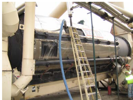
Figure 5 Feeding Advera WMA through Fiber Feed Line
