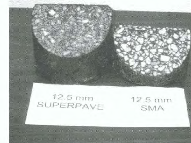
The difference in aggregate structure between dense-graded and SMA is shown in these core samples.
